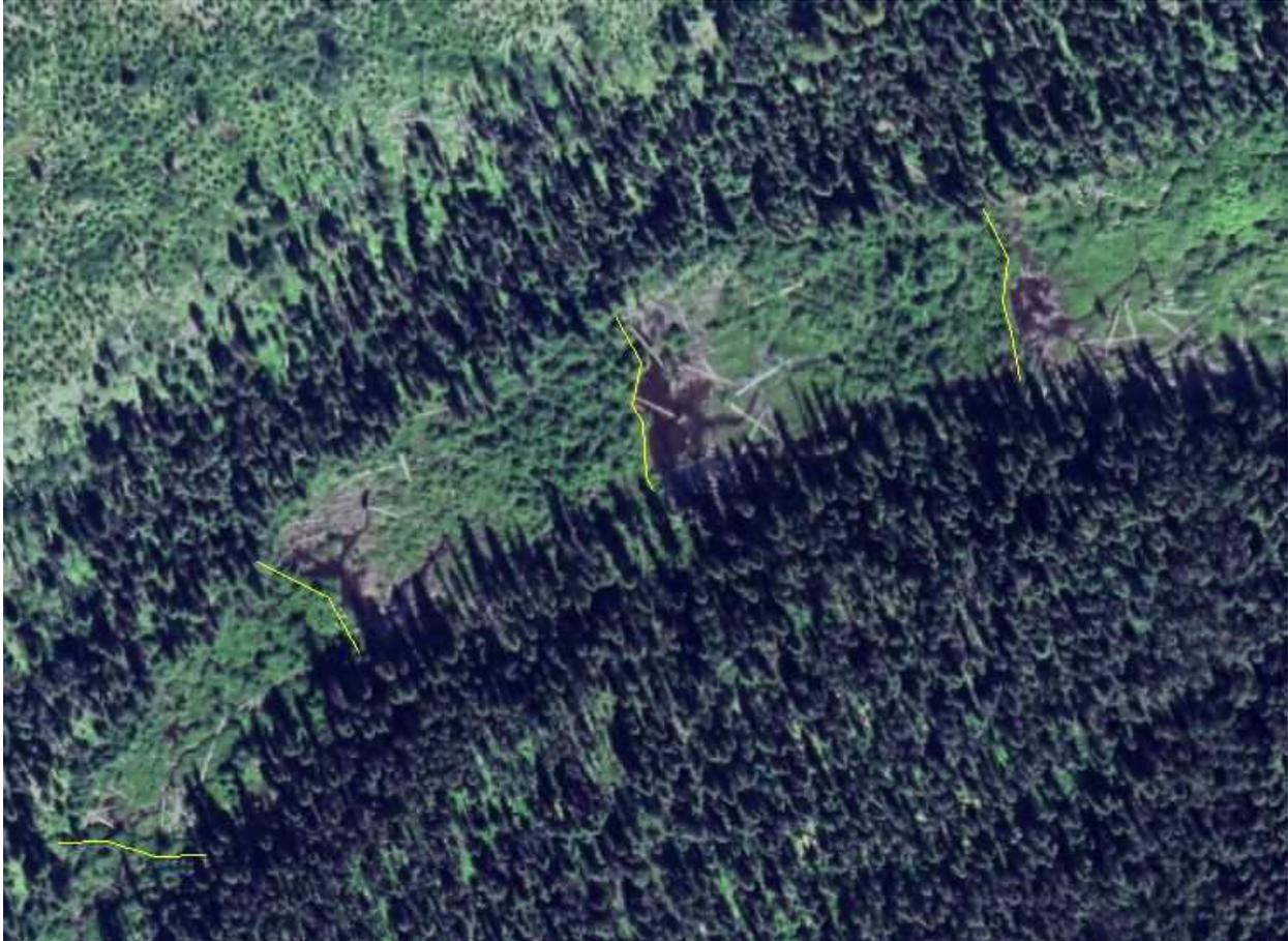
*Figure 1. Four abandoned and breached dams (West arm Kluk Creek), highlighted with yellow lines, appear in this image. Three of the dams have remnants of their former ponds immediately upstream.*
