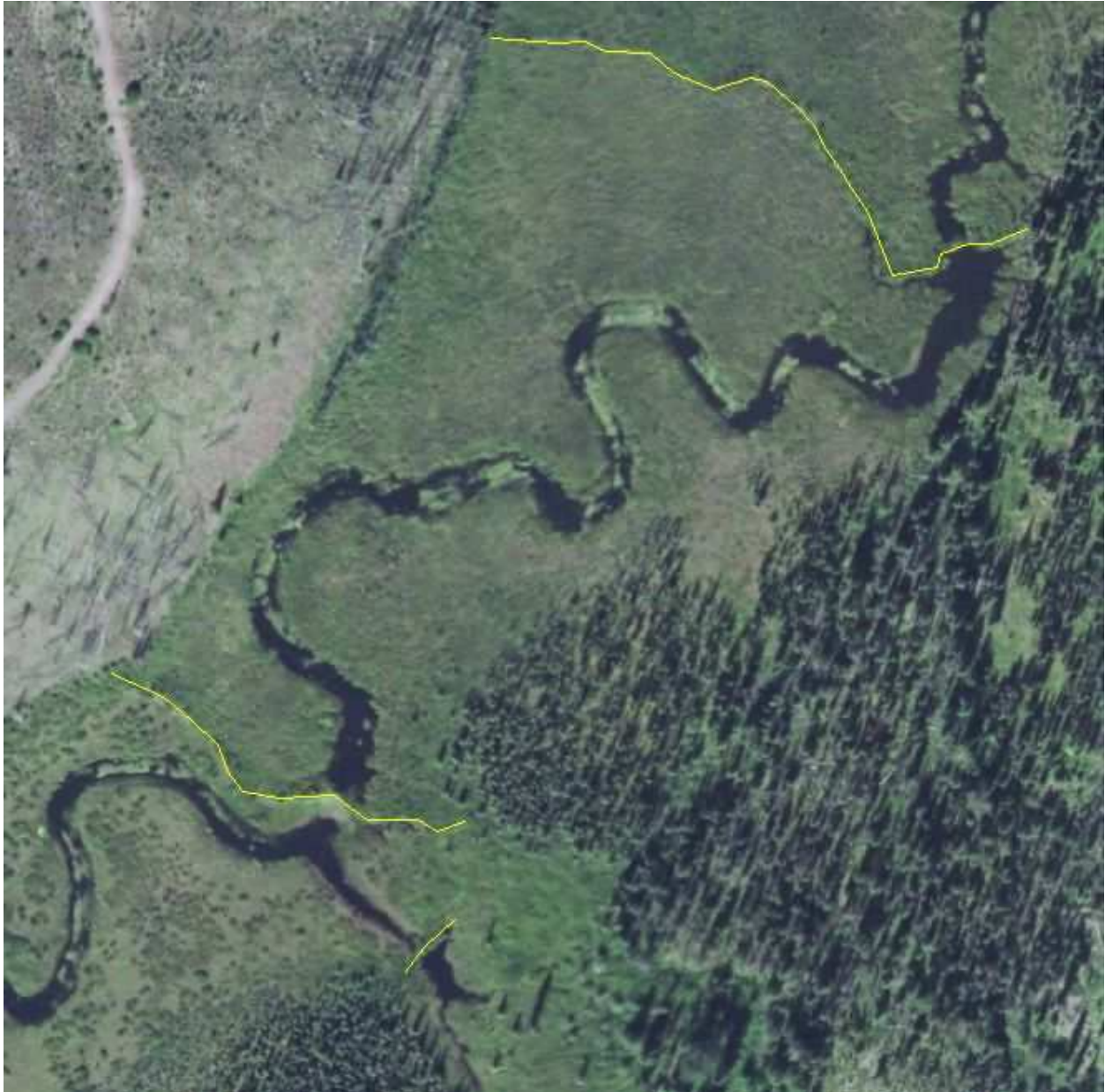
Figure 3. Three old abandoned and breached dams (Cutoff Creek). The longest is about 200 m long. The shortest is across a tributary of the larger channel.
