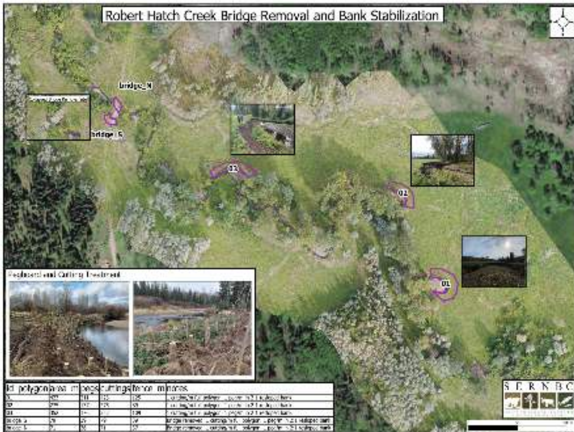
Figure 5.22: Restoration plan for Robert Hatch Creek including removal of collapsed bridge, resloping of banks and the installation of live cuttings/pegboarding
